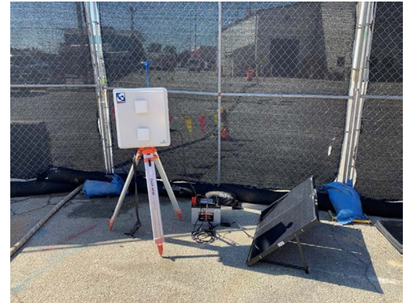
Air monitoring station
