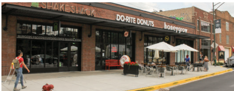
Example of new commercial development on intersecting streets that incorporates flat metal awnings and floor to ceiling window displays, punched through brick facades with hanging placard signage (Lake and Morgan).
