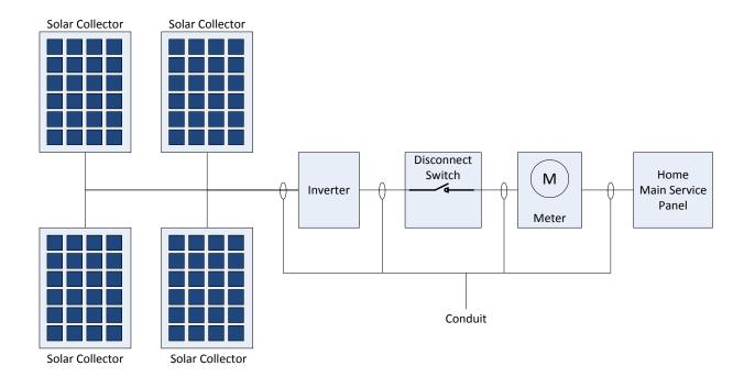
Figure 4: Single Line Diagram of Solar PV System
