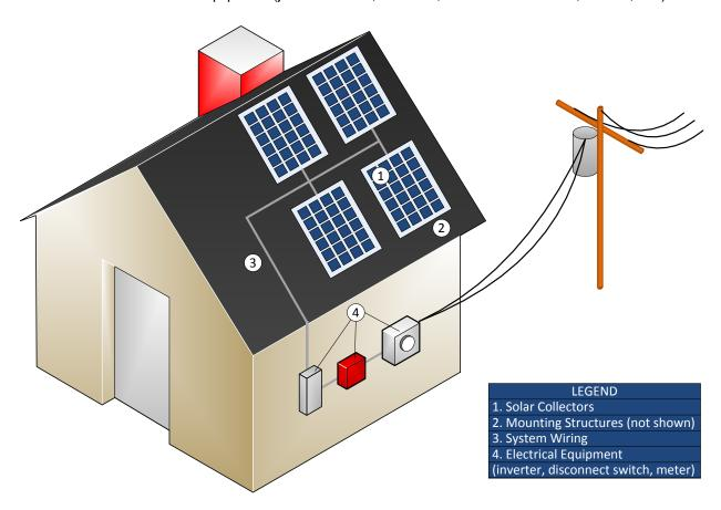
Figure 3: Graphical Illustration of Components for a Typical Rooftop Solar PV System
