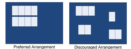
Figure 12: Arrangement solar collectors should be consolidated as much as possible.
