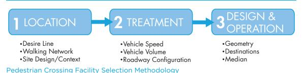
Figure 31 presents a three-step process for locating and designing pedestrian crossing facilities. First, locate the crossing according to the pedestrian network. Second, determine the crossing treatment (signal, refuge island, marked crosswalk). Last, design the crossing and its operation.
