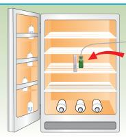
Place the probe of the digital thermometer in the center of the refrigerator.
