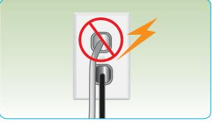
Do not plug more than one appliance into an outlet. This will prevent tripping of circuit breakers.
