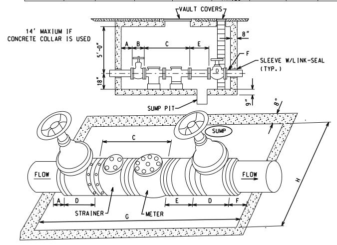
1" TAPS REQUIRED UPSTREAM AND DOWNSTREAM. ALL PIPES AND FITTINGS SHALL BE FLANGED AND SHALL CONFORM TO U.S.A. STANDARD A21.51-1965 (A.W.W.A.C. 151-65) AND SHALL HAVE ON OUTSIDE BITUMINOUS COATING OF EITHER COAL TAR OR ASPHALT BASE AND A CEMENT MORTAR LINING CONFORMING TO U.S.A. STANDARD A21.4-64 (A.W.W.A.C. 104-53).
