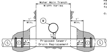
PROFILE THROUGH SEWER/DRAIN
