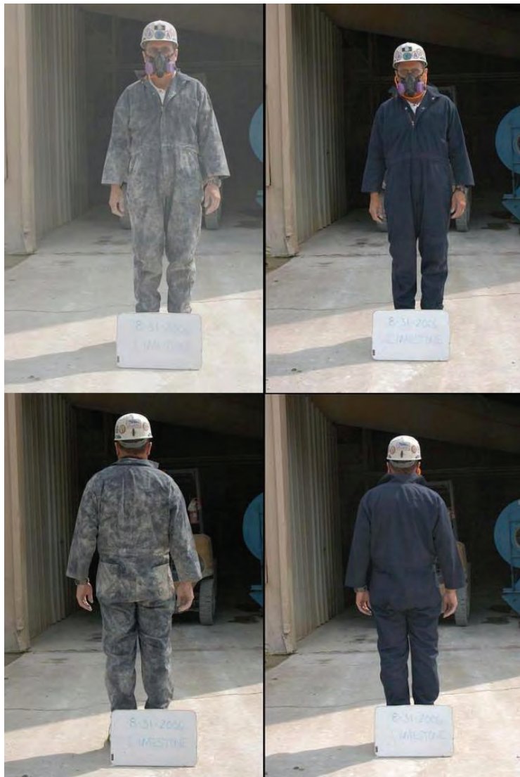
Figure 4-17. Test subject before and after using the clothes cleaning booth.
