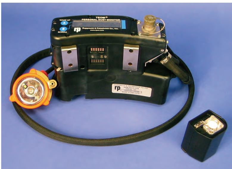
Figure 2-3. Personal dust monitor (PDM) with TEOM unit removed and shown on right.
