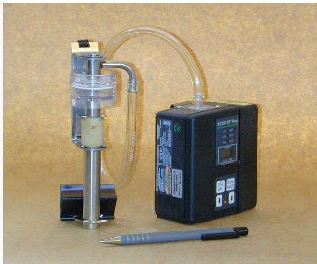
Figure 2-1. Gravimetric sampling pump, cyclone and filter cassette.
