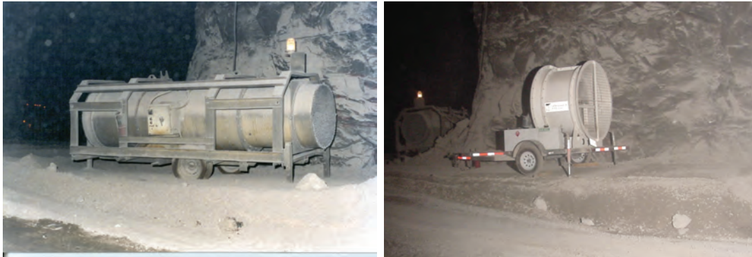
Figure 3-6. Axial vane fan (left) versus propeller fan (right).
