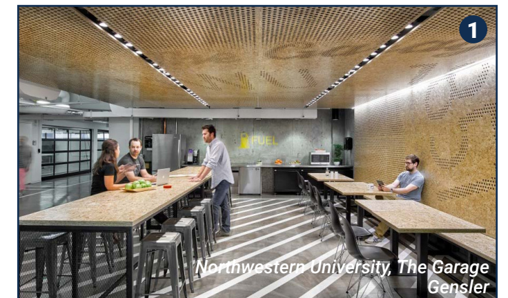
Northwestern University, The Garage Gensler Flat floors and floor-to-floor heights allowed this parking garage to be repurposed as an incubator space.
