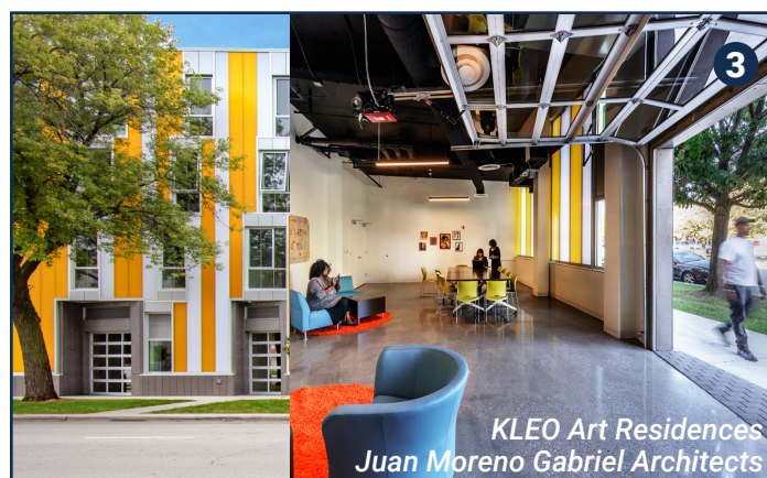
Glass garage doors allow for transparency and easy access into art and community spaces.
