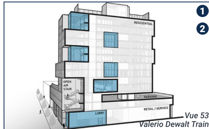
Active ground floor, easy resident access to upper floors, and hidden parking make complementary uses work.
