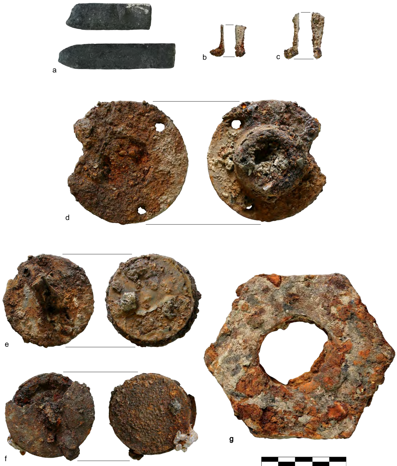
Figure 7.7. Hardware: (a) 11CK1292-HU12A graphite rod from arc lamp; (b–c) 11CK1292-HU12A clips, possibly from arc lamp mechanism; (d) 11CK1292-HU12 iron bracket; (e–f) 11CK1292-HU12 metal closures; 11CK1291-HU10 large nut.
