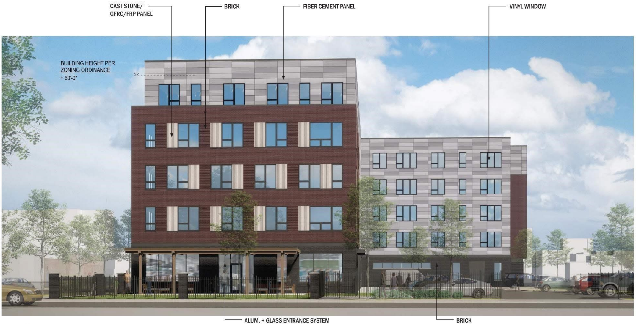
BUILDING ELEVATION (SOUTH)
