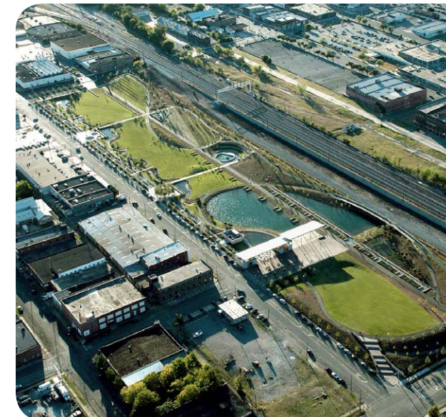
Figure 3: Railroad Park, Birmingham, Alabama, public park on 19 acres of abandoned industrial land, that provides overflow stormwater and flooding zones. Image: Tom Leader Studio
