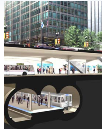
Image 2-11: The East-West Transitway would travel below street level but above the subway lines.
