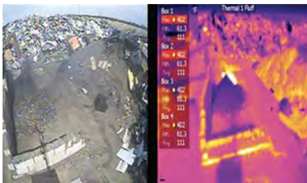
In these side-by-side shots of a recycling yard, the right-hand image shows the bright heat signatures as seen through an infra-red camera.
