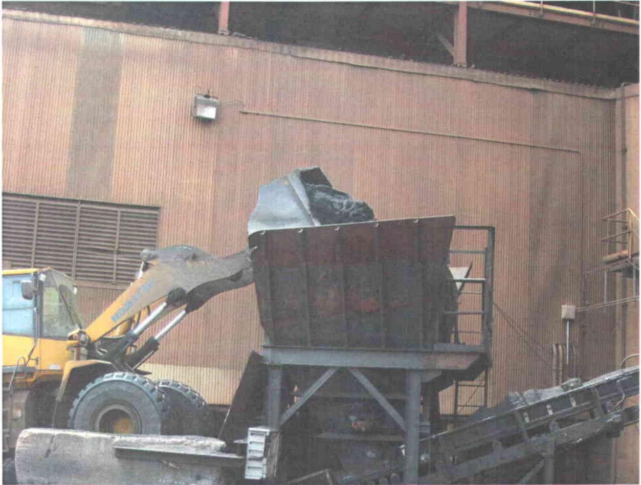
Test 8 – Coke Reclaim Hopper Loading (Informational View 1)
