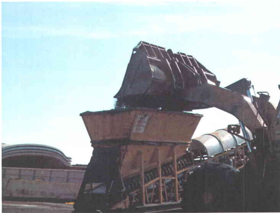
Test 1A – Barge Loading Front End Loader Operation
