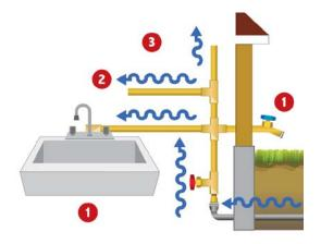
(1) Please find the closest available tap (an outside hose spigot, laundry sink faucet or bathtub) to where the water comes into the home that is not used for drinking water. Fully open the cold water tap and let the water run for at least 5 minutes. Next flush any other cold water faucets on that floor for at least 5 minutes.
