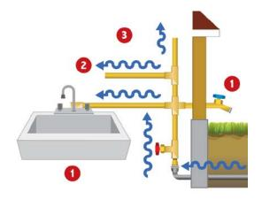
(1) Please find the closest available tap (an outside hose spigot, laundry sink faucet or bathtub) to where the water comes into the home that is not used for drinking water. Fully open the cold water tap and let the water run for at least 5 minutes. Next flush any other cold water faucets on that floor for at least 5 minutes.
