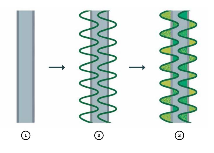
Retrofitting the edges of this channelized waterway into green buffers will help to re-establish the "natural" form and process of the river. By adding vegetated installations to the walls of the canal, floating at its edges, and atop the banks, naturalizing wherever possible, the surface area of the edge is increased, mimicking the lost riparian zone, and bringing back habitat potential and the ability to intercept stormwater from the urban fringe above.
